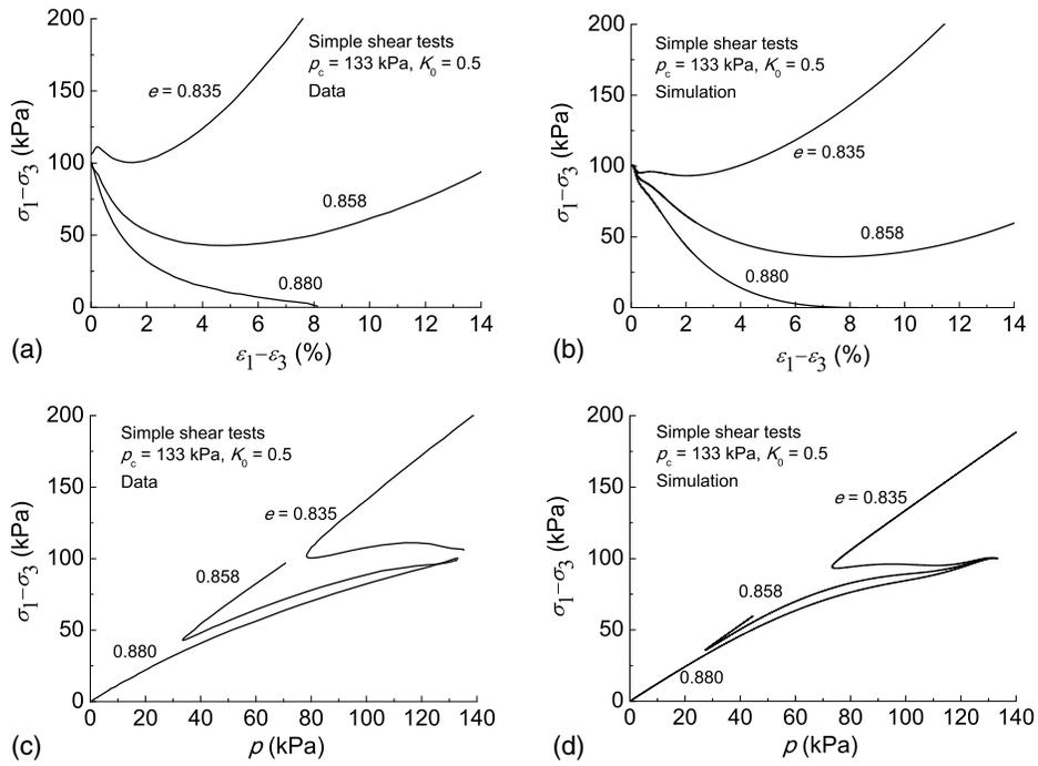
**Fig. 5.** Comparison between model simulations and undrained simple shear test data on Toyoura sand with initially anisotropic stress state (data from Yoshimine et al. 1998)
