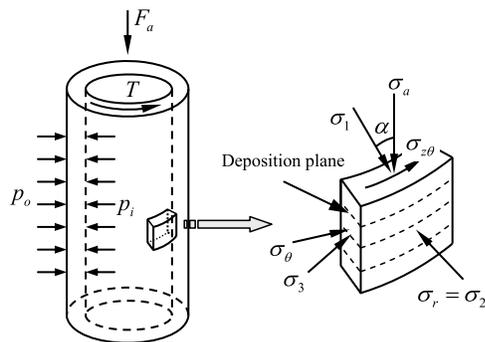
Fig. 2. Torsional shear test setup and stress state for sand element (reprinted from Yoshimine et al. 1998, with permission)
