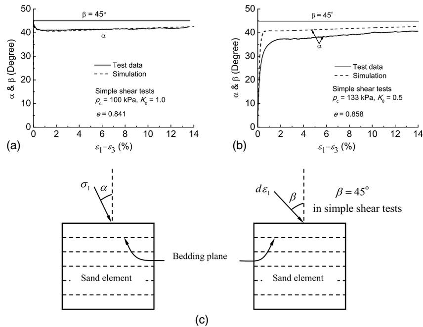
**Fig. 8.** (a) and (b) Comparison between tested and simulated noncoaxial sand response in undrained simple shear tests (data from Yoshimine et al. 1998); (c) illustration of relation between  $\alpha$  and  $\beta$
