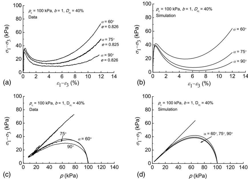
**Fig. 4.** Test data and model simulations for influence of principal stress direction  $\alpha$  on undrained behavior of Toyoura sand at  $b = 1$  (data from Yoshimine et al. 1998)
