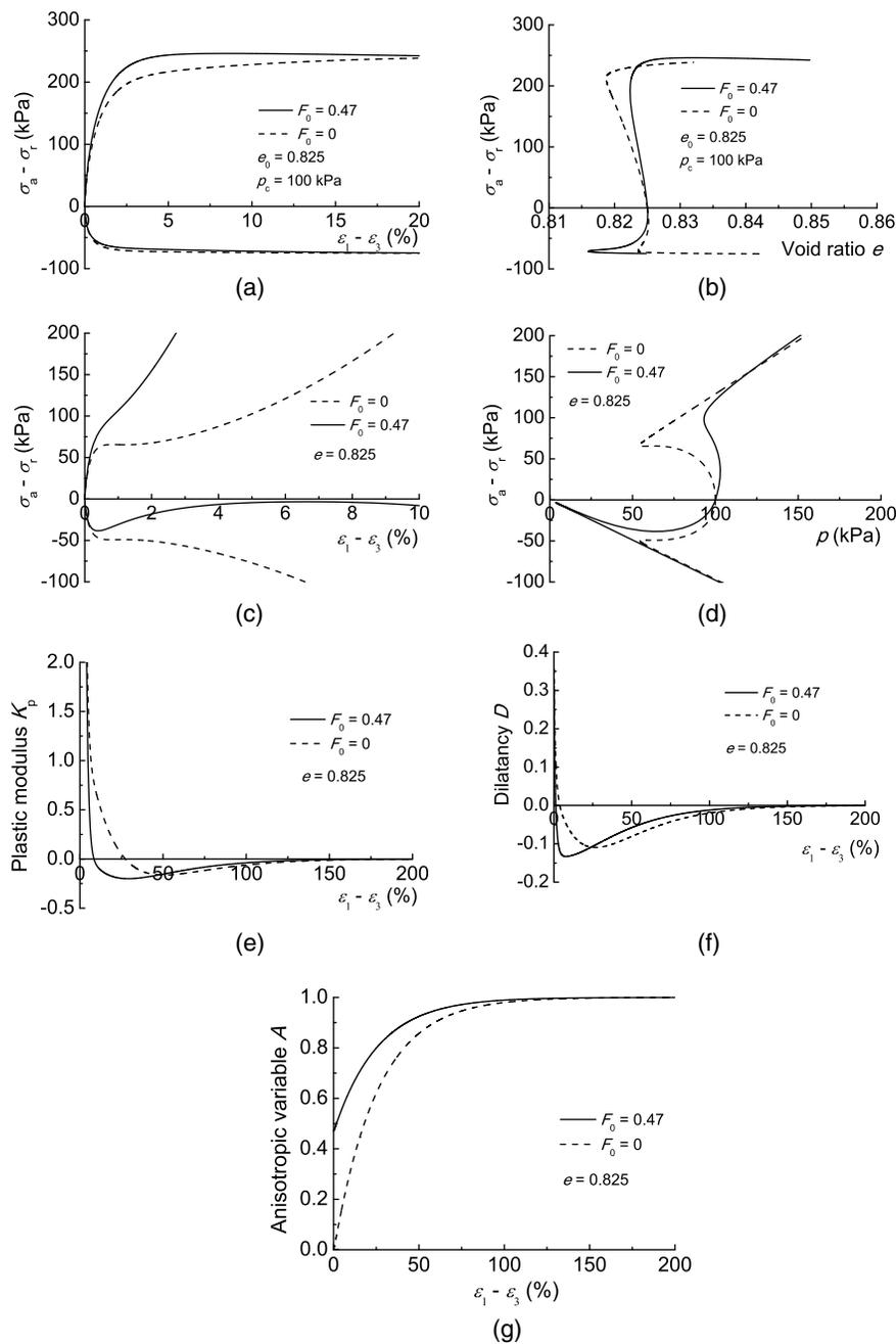
**Fig. 9.** Model simulation for effect of sample preparation method on sand behavior in (a) and (b) drained triaxial tests; (c) and (d) undrained triaxial test; (e)–(g) evolution of  $K_p$ ,  $D$ , and  $A$  for cases with  $F_0 = 1$  and  $0.47$  in drained triaxial compression
