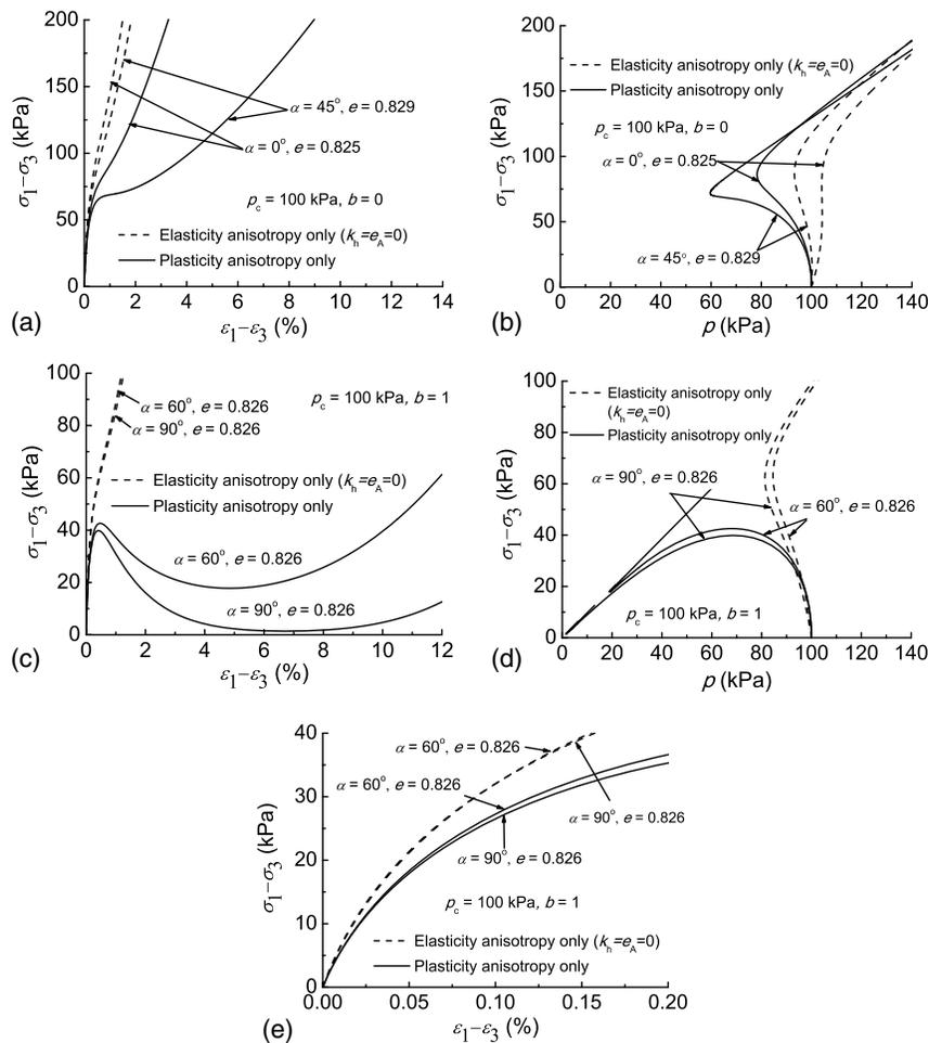
**Fig. 6.** Effect of anisotropic elasticity on model responses in undrained torsional shear tests: (a) and (b)  $b = 0$ ; (c), (d), and (e)  $b = 1$
