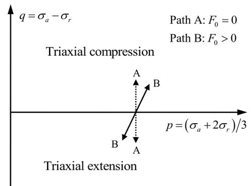
Fig. 1. Stress paths at the very beginning of undrained triaxial tests
