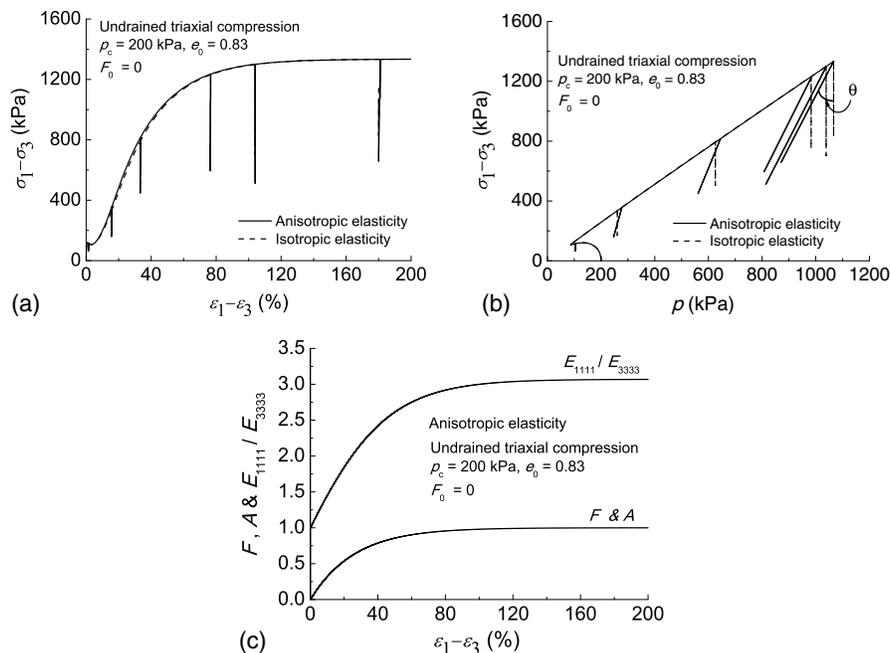
**Fig. 7.** Effect of elasticity anisotropy evolution on sand response in undrained triaxial compression: (a) shear stress-strain relation; (b) effective stress path; (c) evolution of ratio  $E_{1111}/E_{3333}$  with shear strain
