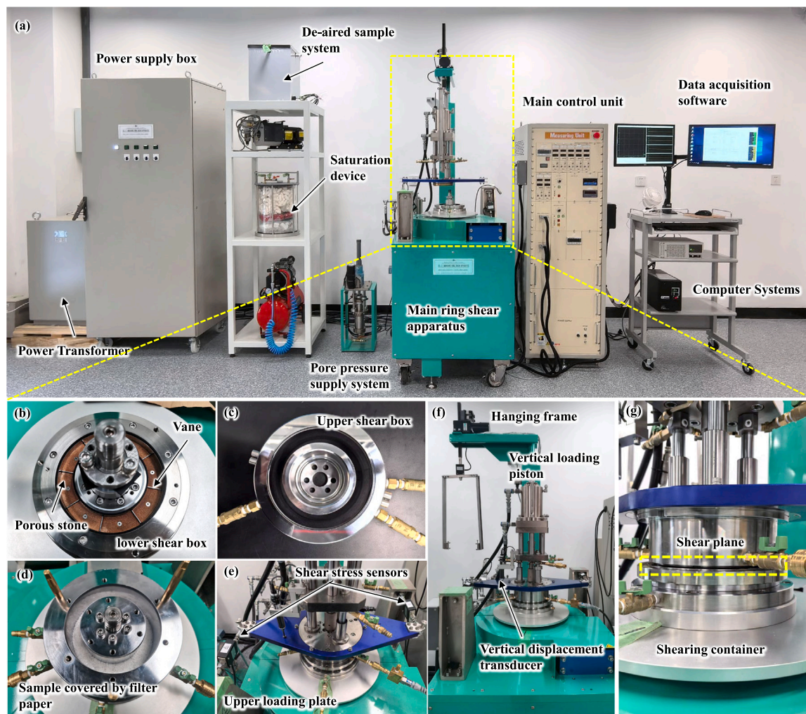
Fig. 2. Undrained high-speed ring shear apparatus used in this study: (a) device composition; (b) lower shear box; (c) upper shear box; (d) sample setting process; (e) connection to normal stress loading system; (f) hanging frame for lifting of loading cap; (g) position of shearing plane during test.
