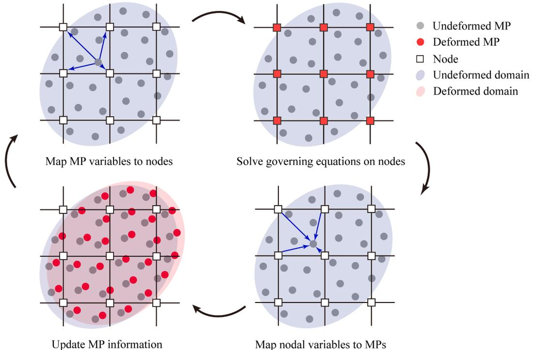
Fig. 1. Illustration of typical MPM procedure.
