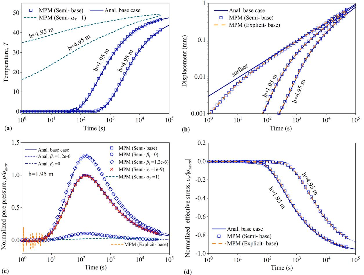
**Fig. 5.** MPM solutions against analytical solutions for the 1D heating of a saturated half-space: (a) temperature versus time, (b) surface displacement versus time, (c) normalized pore pressure  $p/p_{max}$  versus time, in which  $p_{max}$  is the maximum pore pressure in the base case, and (d) normalized effective stress  $\sigma_x/|\sigma_{xmax}|$  versus time, in which  $\sigma_{xmax}$  is the maximum lateral stress.
