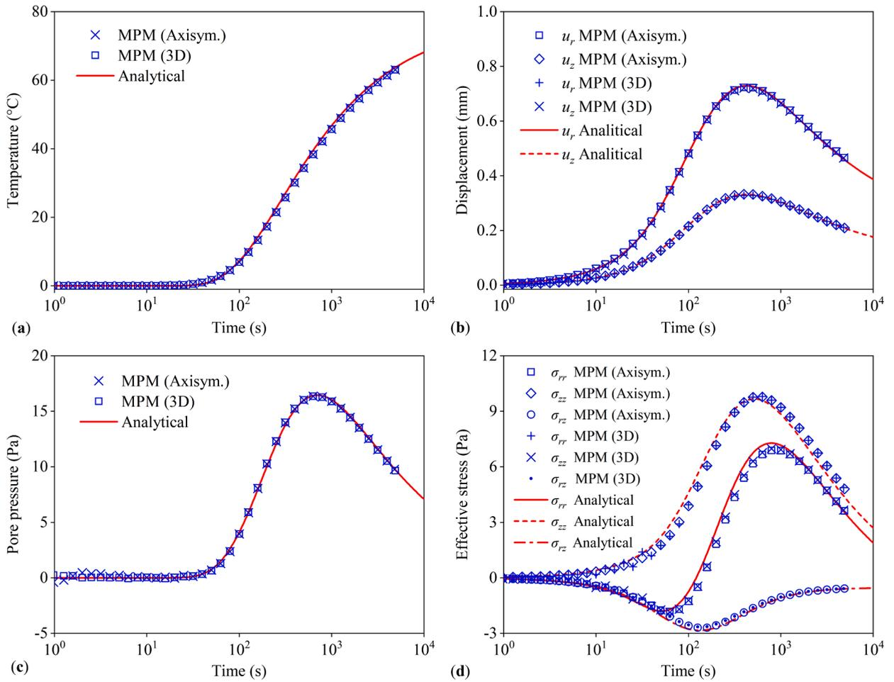
**Fig. 14.** MPM results against analytical solutions: (a) temperature, (b) displacement components  $u_r$  and  $u_z$ , (c) pore pressure, and (d) effective stress components  $\sigma_{rr}$ ,  $\sigma_{zz}$ , and  $\sigma_{rz}$  as a function of time at point (0.561041 m, 0.25531 m, 0 m).
