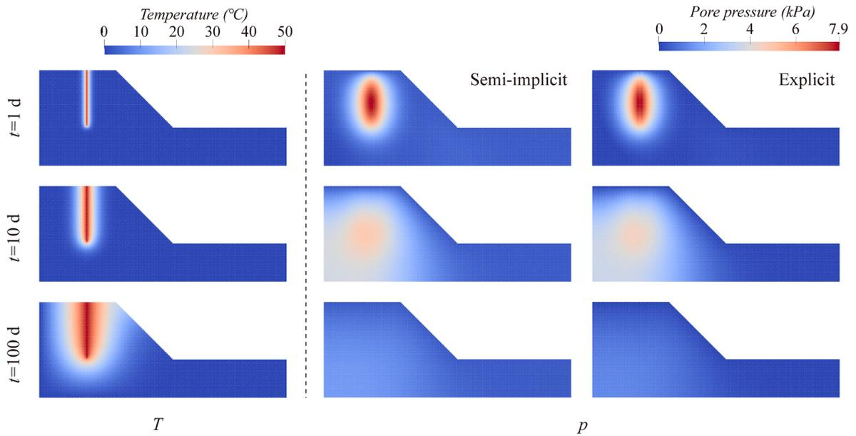
Fig. 20. Temperature and pore pressure fields at different time instances during the heating process for both the semi-implicit and explicit MPM.
