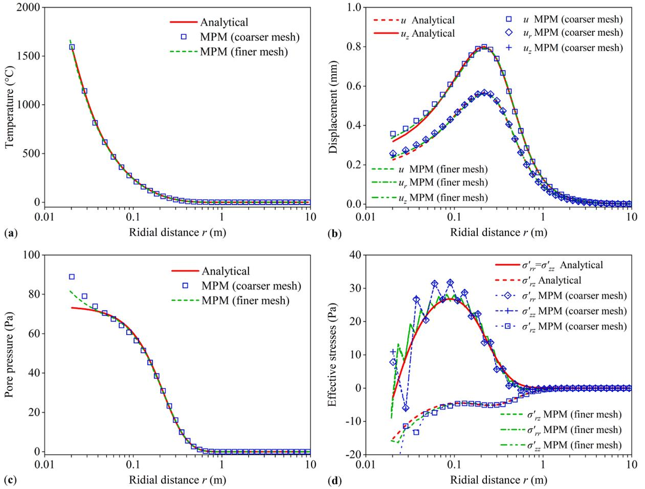
Fig. 15. Spatial distribution of (a) temperature, (b) displacement components  $u_r$  and  $u_z$ , (c) pore pressure, (d) effective stress components  $\sigma'_{rr}$ ,  $\sigma'_{zz}$ , and  $\sigma'_{rz}$  along the 45-degree line at  $t = 100$  s. (For interpretation of the references to color in this figure legend, the reader is referred to the web version of this article.)
