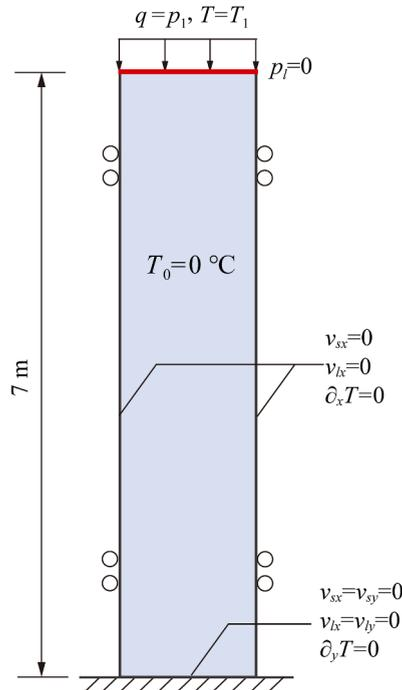
Fig. 7. Geometry and boundary conditions for non-isothermal consolidation.
