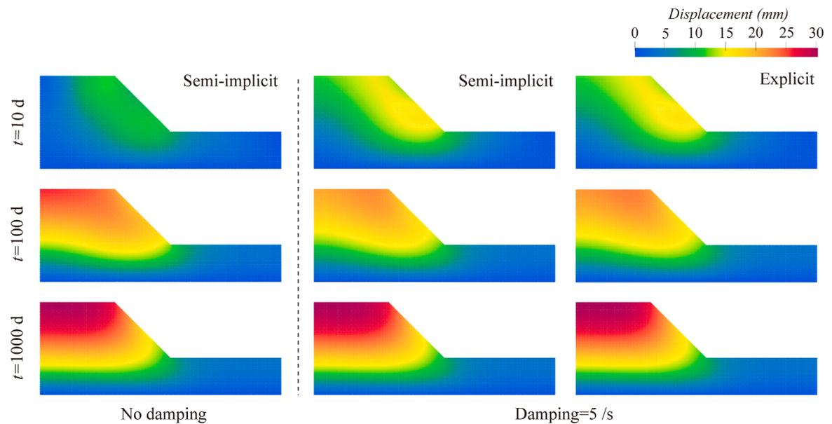
Fig. 18. Comparison of the displacement field for semi-implicit MPM and explicit MPM with and without damping at different time instances during the gravity loading.
