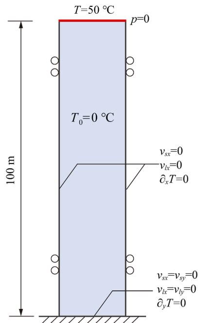
Fig. 4. Geometry and boundary conditions for 1D heating.
