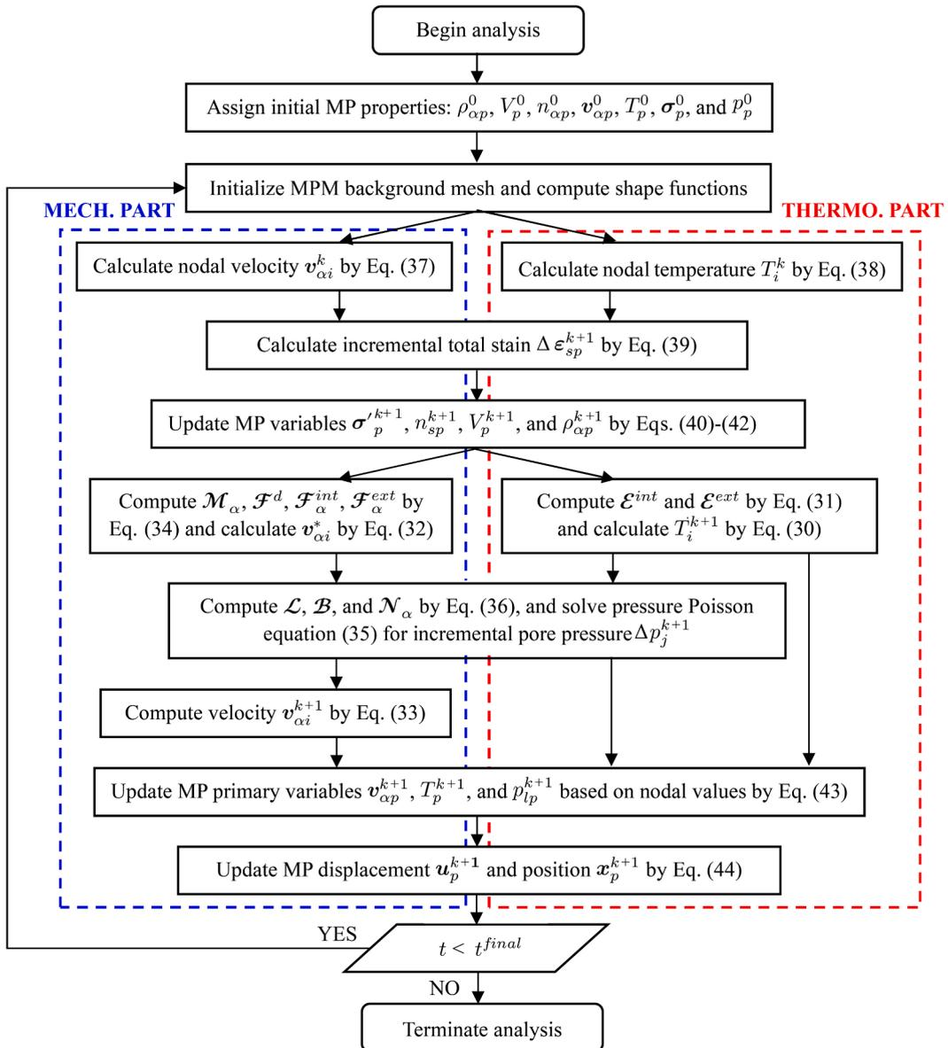
Fig. 2. Solution procedure of the semi-implicit THM-coupled MPM.
