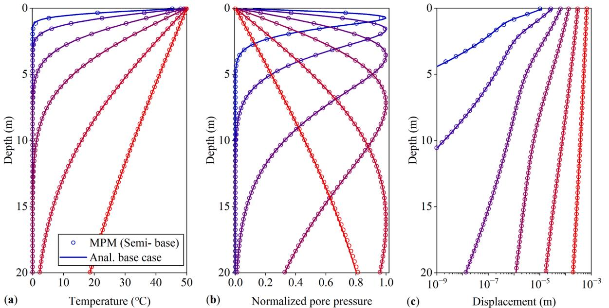
Fig. 6. Spatial distributions of (a) temperature, (b) pore pressure, and (c) displacement at different time instances:  $t = 20 \text{ s}, 100 \text{ s}, 500 \text{ s}, 2000 \text{ s}, 10000 \text{ s},$  and  $50000 \text{ s}$ , represented by lines from up (blue) to bottom (red), respectively. (For interpretation of the references to color in this figure legend, the reader is referred to the web version of this article.)
