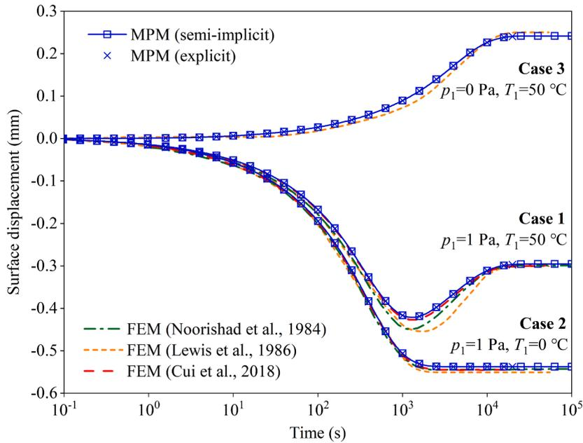
Fig. 10. Surface settlement versus time for both non-isothermal and isothermal conditions.
