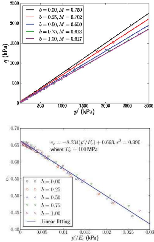
FIGURE 2. DEM data for the critical stress ratio (upper) and the critical state void ratio (bottom) and fittings.
