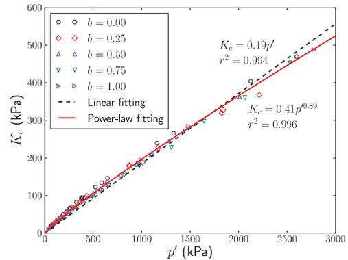
FIGURE 4. Correlation between the critical state values of the first joint invariant  $K$  with the mean effective stress  $p'$ .
