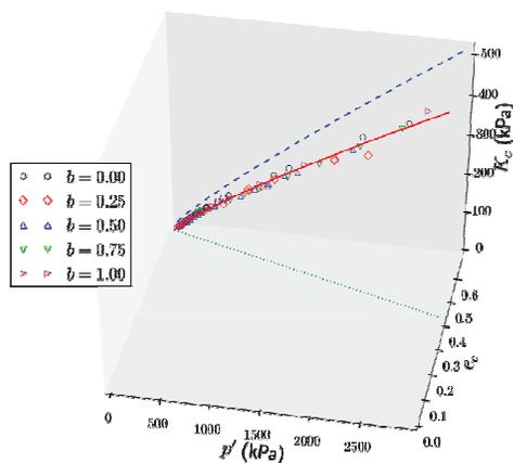
FIGURE 6. A unique critical state curve plotted in the space of  $K$ - $e$ - $p'$ .
