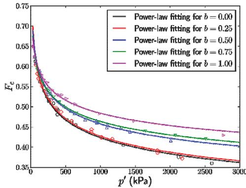
FIGURE 3. Correlation between the critical fabric anisotropy  $F_c$  (defined by the second invariant of  $F_{ij}$ ) with the mean effective stress  $p'$ .
