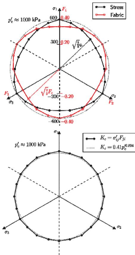
FIGURE 5. State surfaces of critical state stress and critical fabric anisotropy in the deviatoric plane (upper) and  $K_c$  in the deviatoric plane at  $p'_c = 1000$  kPa.
