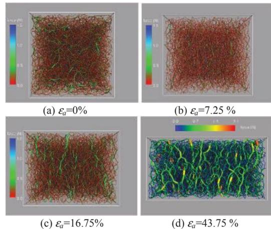
**FIGURE 1.** The evolution of fabric structure in a medium dense granular assembly subjected to undrained shear from an initial isotropic state (a) to the critical state (d), obtained by DEM simulations. The columns in the figure denote the contact normal force chain developed at particle contacts. The thickness of each column represents its magnitude.
