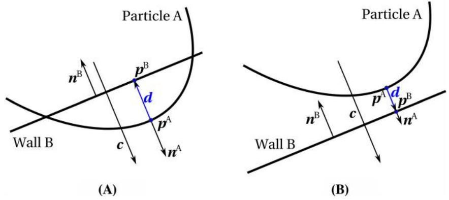
**FIGURE 9** Two-dimensional schematic of the contact quantities for A, contacting and B, noncontacting particle-wall pairs [Colour figure can be viewed at [wileyonlinelibrary.com](http://wileyonlinelibrary.com)]
