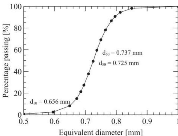
**FIGURE 23** Grain size distribution of numerical specimens
