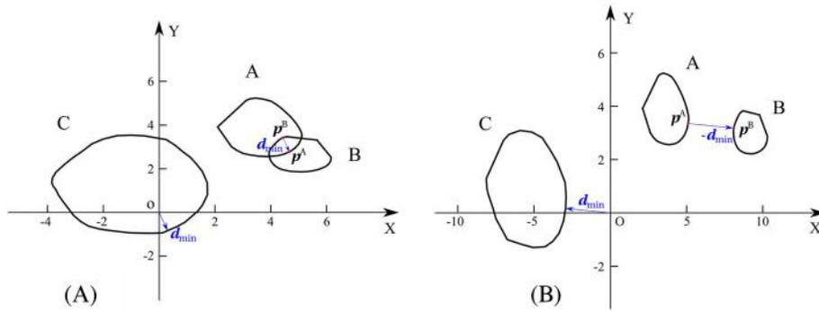
**FIGURE 10** Two-dimensional schematic of Minkowski difference  $C$  of two arbitrary convex particles  $A$  and  $B$ , with or without contact [Colour figure can be viewed at [wileyonlinelibrary.com](http://wileyonlinelibrary.com)]
