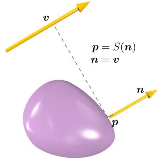
**FIGURE 6** A support point  $\mathbf{p}$  on a particle surface with a given direction vector  $\mathbf{v}$  and a support function  $S(\mathbf{n})$ . Note:  $\mathbf{n}$  is the outward normal of particle surface at the support point  $\mathbf{p}$  [Colour figure can be viewed at [wileyonlinelibrary.com](http://wileyonlinelibrary.com)]
