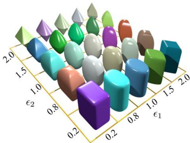
**FIGURE 1** Superellipsoids with  $r_x = 1.0$ ,  $r_y = 1.5$ ,  $r_z = 2$  and varying  $\epsilon_1$  and  $\epsilon_2$  [Colour figure can be viewed at [wileyonlinelibrary.com](http://wileyonlinelibrary.com)]
