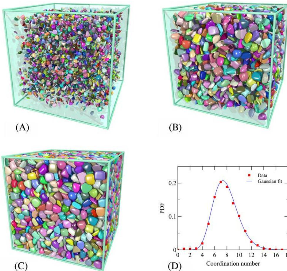
**FIGURE 21** A, Initial packing with randomly positioned particles; B, packing after particles expand to the target size; C, packing after isotropic consolidation; D, probability distribution function (PDF) of coordination number within the packing in (C) [Colour figure can be viewed at [wileyonlinelibrary.com](http://wileyonlinelibrary.com)]
