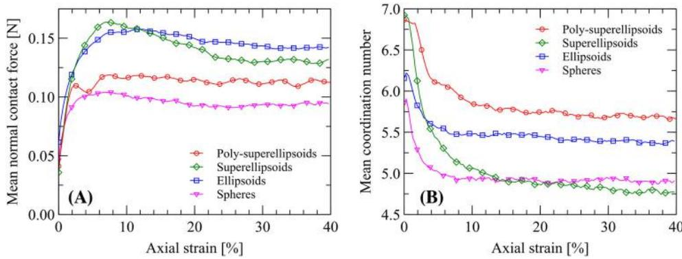
**FIGURE 26** Evolution of A, mean normal contact force and B, mean coordination number for specimens with different particle shapes during shearing [Colour figure can be viewed at [wileyonlinelibrary.com](http://wileyonlinelibrary.com)]
