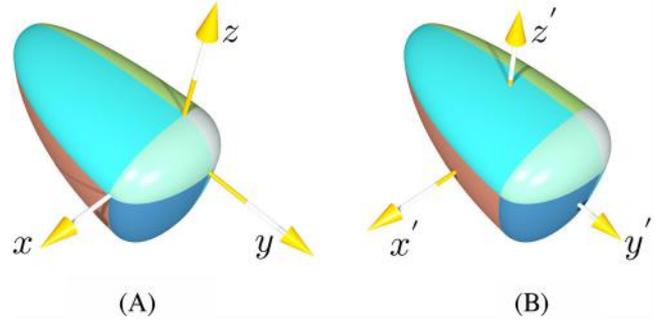
**FIGURE 3** Poly-superellipsoids with  $r_x^+ = 1.0, r_x^- = 0.5, r_y^+ = 0.8, r_y^- = 0.9, r_z^+ = 0.4, r_z^- = 0.6$  and A,  $\epsilon_1 = 0.4, \epsilon_2 = 1.5$ , B,  $\epsilon_1 = \epsilon_2 = 1.0$ , C,  $\epsilon_1 = \epsilon_2 = 1.5$  [Colour figure can be viewed at [wileyonlinelibrary.com](http://wileyonlinelibrary.com)]
