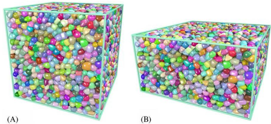
**FIGURE 24** Configurations of the specimen with poly-superellipsoids at A, the initial and B, the final states. Color is for tracking particle movement intuitively [Colour figure can be viewed at [wileyonlinelibrary.com](http://wileyonlinelibrary.com)]
