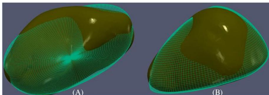
**FIGURE 5** Examples of realistic particles (solid) fitted by poly-superellipsoids (wireframe) with A,  $\epsilon_1 = 0.85, \epsilon_2 = 1.0, r_x^+ = 3.26, r_x^- = 2.67, r_y^+ = 1.66, r_y^- = 1.59, r_z^+ = 1.81, r_z^- = 1.67$  and B,  $\epsilon_1 = 1.1, \epsilon_2 = 1.2, r_x^+ = 2.07, r_x^- = 1.02, r_y^+ = 1.26, r_y^- = 1.23, r_z^+ = 1.40, r_z^- = 0.35$  [Colour figure can be viewed at [wileyonlinelibrary.com](http://wileyonlinelibrary.com)]
