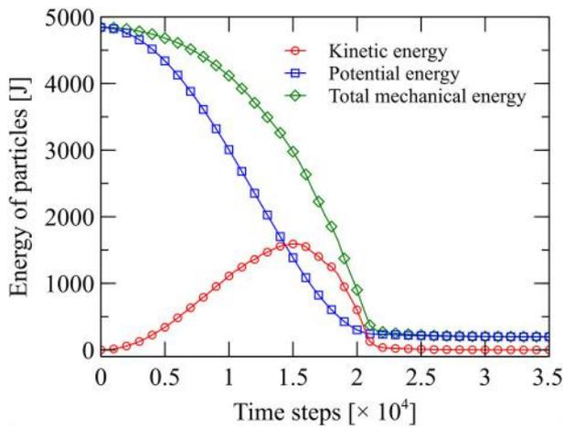
**FIGURE 20** Variations of kinetic, potential, and total energy of particles during the packing [Colour figure can be viewed at [wileyonlinelibrary.com](http://wileyonlinelibrary.com)]
