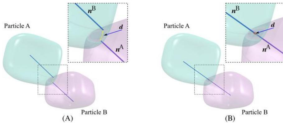
**FIGURE 18** Example of two particles with a flat contact: A, the Levenberg-Marquardt (LM) algorithm fails due to slow convergence after 23 calls of the support function; B, the Gilbert-Johnson-Keerthi (GJK) algorithm succeeds after 12 calls of the support function. Note that the initial guess of the contact normal is the vector joining the mass centers of the two particles [Colour figure can be viewed at wileyonlinelibrary.com]
