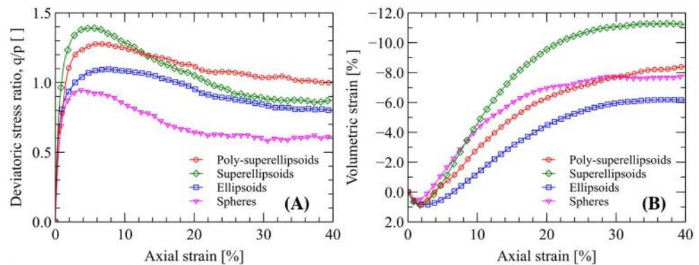
**FIGURE 25** Evolution of A, deviatoric stress ratio  $q/p$  and B, volumetric strain for specimens with different particle shapes during shearing [Colour figure can be viewed at [wileyonlinelibrary.com](http://wileyonlinelibrary.com)]
