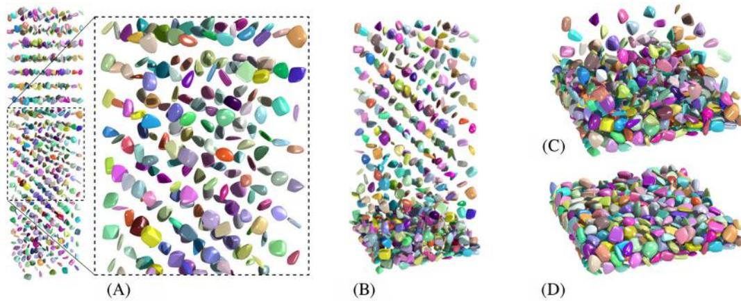
**FIGURE 19** Five hundred poly-superellipsoids falling under gravity: A, initial packing, B, after 15 000 time steps, C, after 20 000 time steps, D, after 35 000 time steps. Note: The box is not shown for a better visualization [Colour figure can be viewed at [wileyonlinelibrary.com](http://wileyonlinelibrary.com)]
