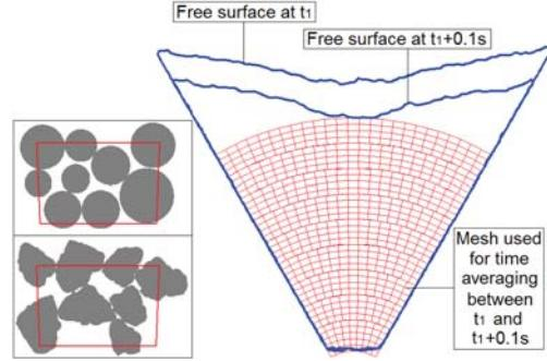
**FIGURE 2.** Mesh used for time averaging between instants  $t_1$  and  $t_1+0.1s$ . The free-surface corresponds to Simulation B. The insert shows typical particles belonging to a given cell.
