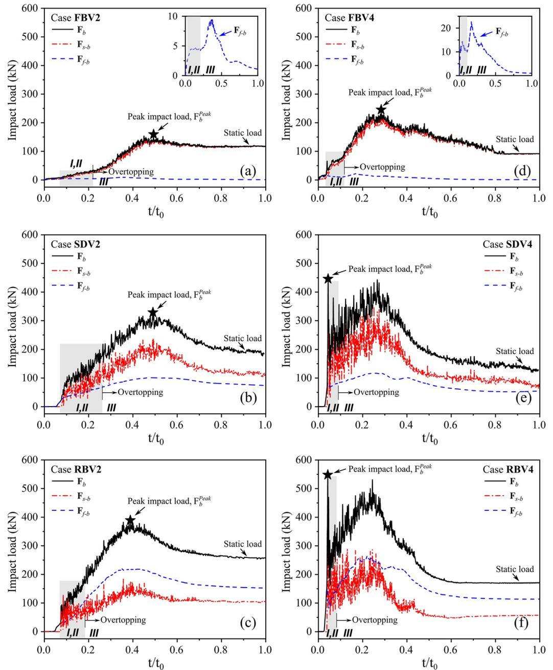
**Figure 6.** Evolutions of the solid-barrier contact force  $F_{s-b}$ , the fluid-barrier interaction force  $F_{f-b}$ , and total impact load  $F_b$  under pile-up (a, b, and c;  $v_{\text{init}} = 2$  m/s) and runup (d, e, and f;  $v_{\text{init}} = 4$  m/s) modes for flexible, slit, and rigid barriers in intercepting two-phase geophysical flows. The gray regions represent the impact durations for stages I and II.
