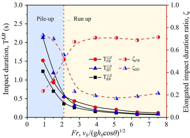
**Figure 8.** Measured relationships of  $Fr$ ,  $T^{I,II}$ , and  $\zeta$  for geophysical flows against flexible, slit, and rigid barriers. The blue and yellow regions represent the pile-up and runup impact modes, respectively.
