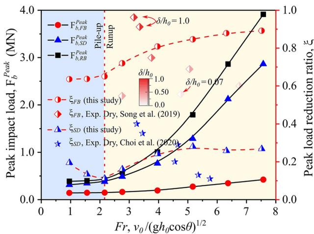
**Figure 7.** Measured relationships between  $Fr$ ,  $F_b^{\text{Peak}}$ , and  $\xi$  for geophysical flows against flexible, slit, and rigid barriers. The blue and yellow regions denote the pile-up and runup impact modes, respectively. The color of half-solid diamonds represent the normalized boulder diameter  $\delta/h_0$  of impinging flows performed by Song et al. (2019).
