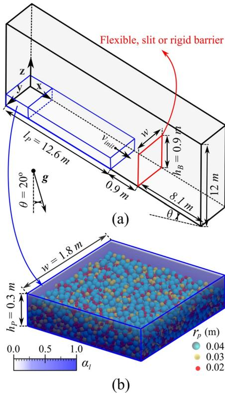
**Figure 3.** Model setup. (a) Model geometry prior to the release of the solid-liquid mixture; and (b) illustration of a representative part of a mixture sample consisting of tridisperse particles and a viscous liquid.  $r_p$  and  $\alpha_l$  denote particle radius and liquid volume fraction, respectively.
