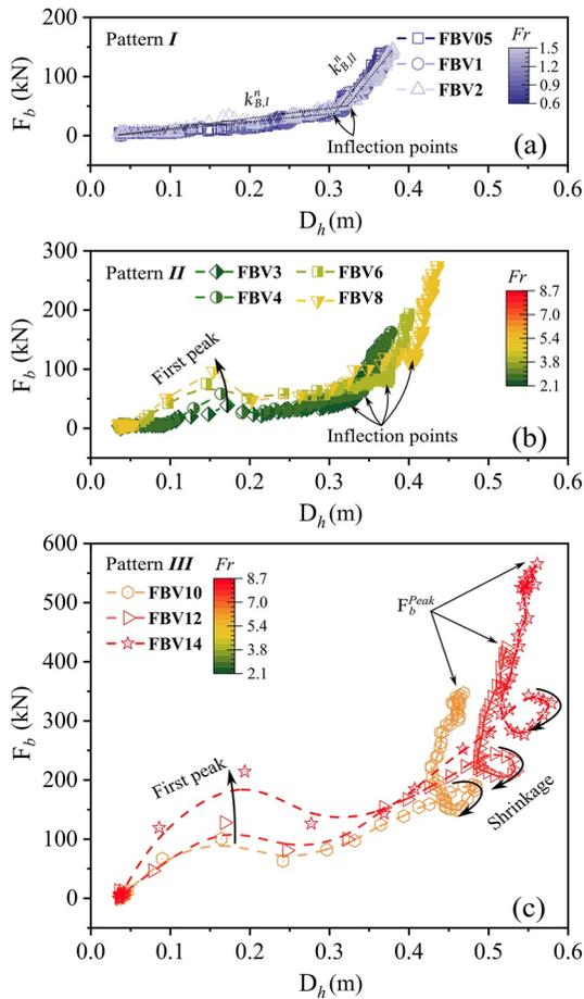
**Figure 9.** The  $Fr$ -dependent load-deformation ( $F_b$ - $D_h$ ) relations of a flexible ring net barrier in arresting geophysical flows for (a) pattern *I*, (b) pattern *II*, and (c) pattern *III*.  $F_b$  and  $D_h$  denote the flow-direction impact load sustained by the barrier and the maximum flow-direction barrier deflection, respectively.
